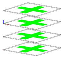
2) Select = Auto, Validity = +Z Validity = -Z (Attention: The free surface load is placed exactly IN the plane of the 3<sup>rd</sup> plate.)
