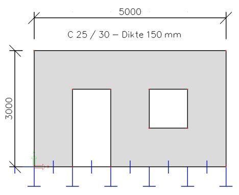
\*Input wall Structure > 2D Member > Plate Structure > 2D Member > 2D member components > Opening
