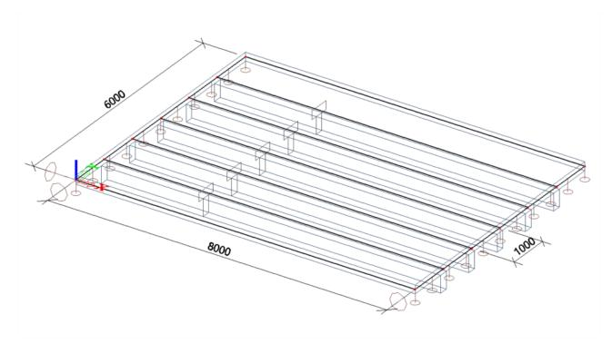
\*Input plate + ribs (Method 1): Structure > 2D Member > Plate
