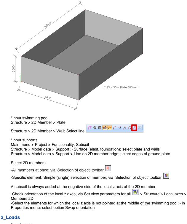
\*Load cases LC 1: Self weight LC 2: Water pressure (Var.) > Surface load 0 to 25 kN/m<sup>2</sup>
