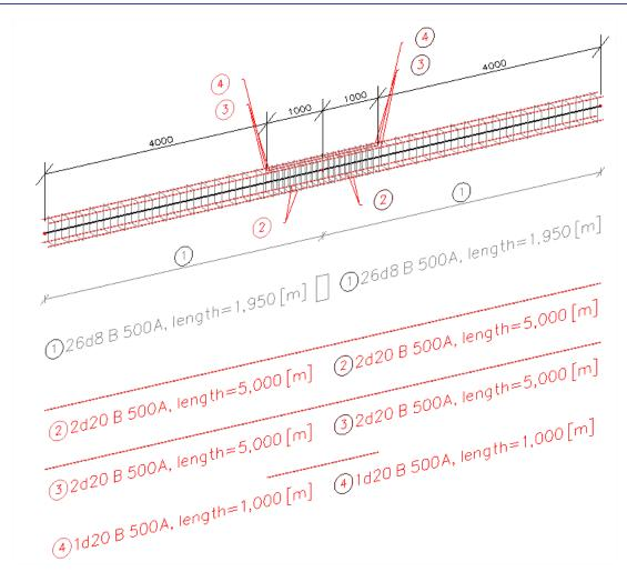
\*Longitudinal reinforcement window:
