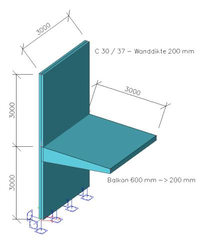
\*Input balcony Structure > 2D Member > Wall Structure > 2D Member > Plate; Thickness type = Variable, Member system plane at = Top
