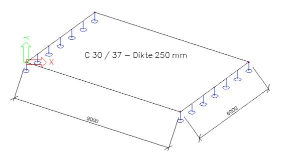
\*Input plate: Structure menu > 2D Member > Plate New rectangle, via Command line toolbar a diagonal of the rectangle; define the 2 nodes on
